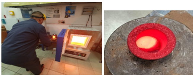
Fig. 3. Reductive smelting of ore-lime briquettes to produce metallic iron and slag.
