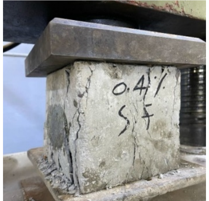
Fig. 9. Crushed concrete cube after the compressive strength test.
