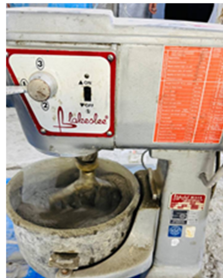
Fig. 3. Electrically operated mechanical mixer.
