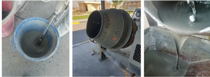
Fig. 4. Slurry mixing process.
