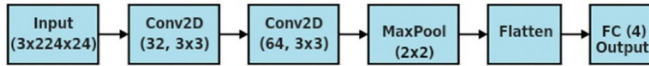
Fig. 2. Architecture of a CNN showing convolution, pooling, and fully connected (dense) layers.
