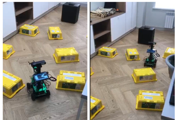
Fig. 8. Mobile robot navigation using an integrated 3D LiDAR system.
