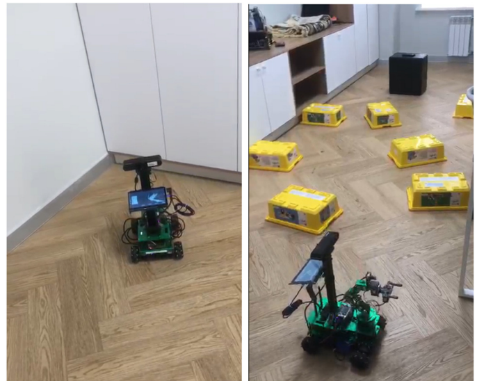
Fig. 7. Mobile robot navigation using a 3D LiDAR sensor.
