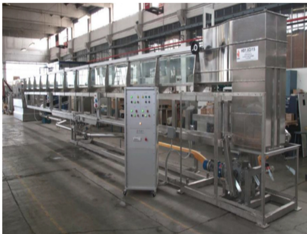
Fig. 2. The laboratory flume.
