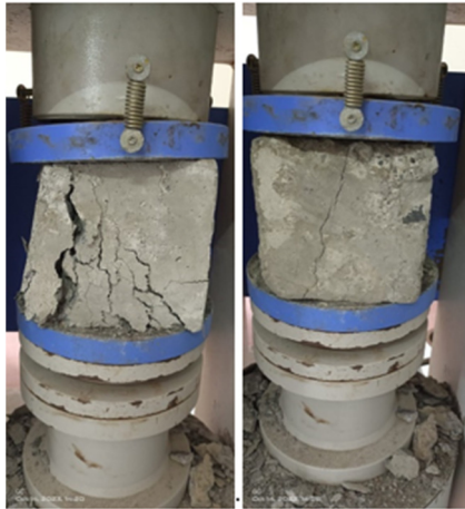
Fig. 4. Concrete cube testing under CTM.
