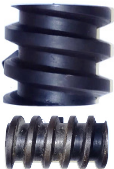
Fig. 15. Designs of screw sections of various lengths for the extruder.
