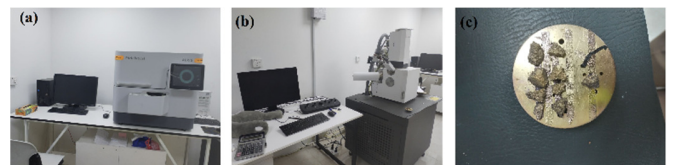
Fig. 4. (a) The XRD equipment, (b) the SEM instrument, and (c) the mounted SCC samples for SEM characterization.
