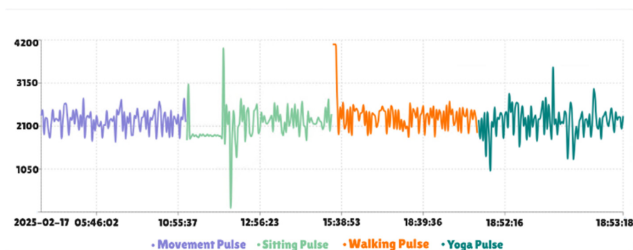
Fig. 13. Dynamics of raw PPG sensor readings over time. The y-axis represents unprocessed signal amplitude, not beats per minute (BPM).
