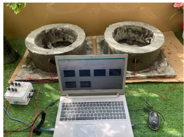
Fig. 2. Schliebinger system for restrained drying shrinkage testing.
