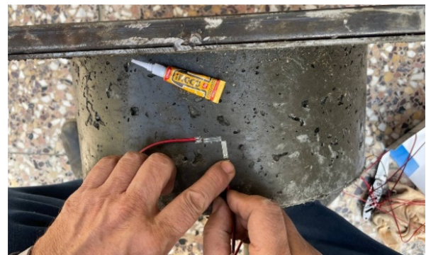
Fig. 1. Strain gauge fixing on restrained concrete sample.
