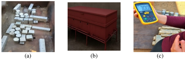
Fig. 4. Burning process. (a) Placing the specimens in the furnace, (b) burning furnace, (c) digital thermometer.
