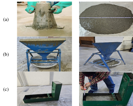
Fig. 3. Fresh tests. (a) Slump flow test, (b) V-funnel test, (c) L- Box test.
