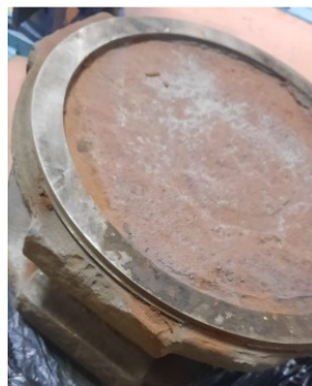
Fig. 2. The worn part of the wedge.
