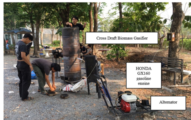
Fig. 1. Imbert-type cross draft gasifier experimental setup.
