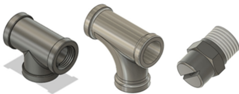
Fig. 3. Geometry of regular Tee, Tee Y, and Flat Fan Nozzle (left to right).
