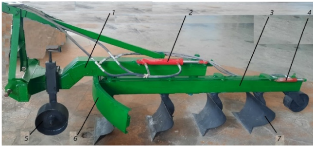
Fig. 1. (1) Dump plough configuration consisting of the main frame, (2) hydraulic cylinder for frame rotation, (3) rotating frame, (4) hydraulic cylinder for working parts' rotation, (5) support wheel, (6) guide arc, and (7) diamond-shaped plough.
