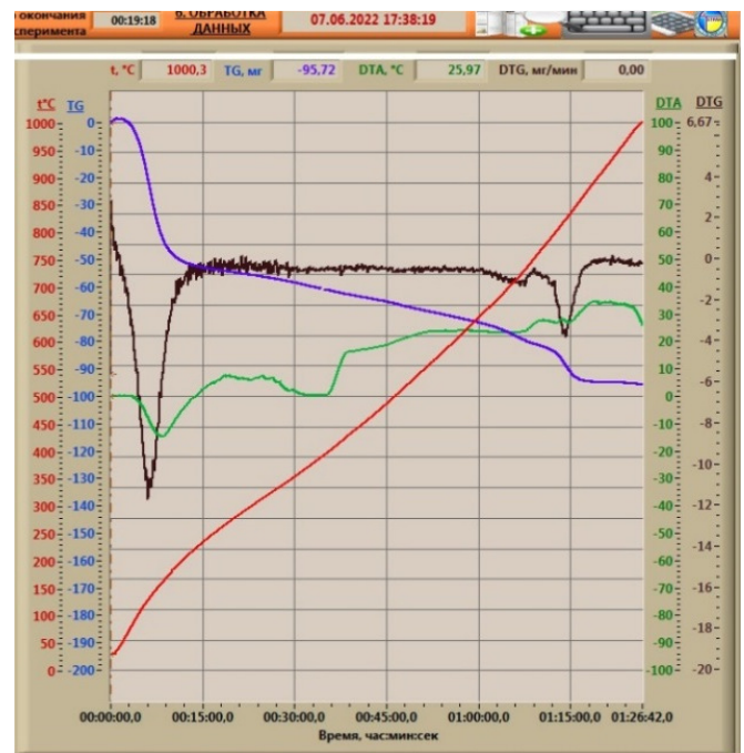
Fig. 1. DTA of Darbaza clay suspension with 0.5% polymer reagent.
