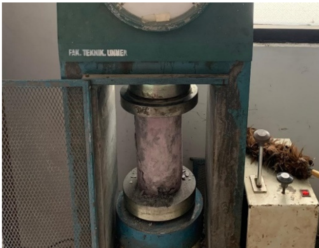
Fig. 8. Compressive strength test setup.
