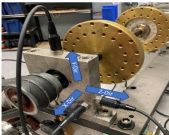
Fig. 2. Perpendicular installation of sensors on bearing 1.
