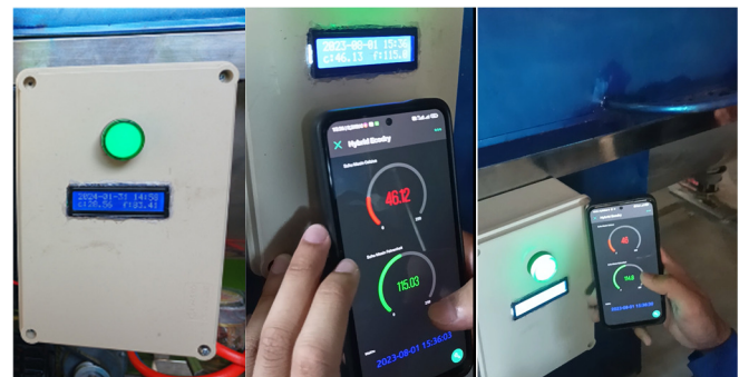
Fig. 5. Integrating an IoT system with a drying machine.
