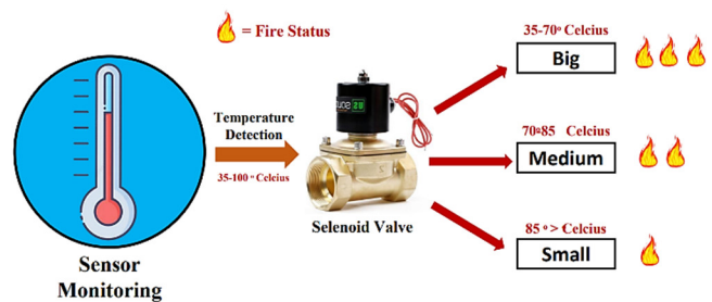
Fig. 7. Gas solenoid valve work scheme.
