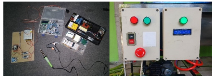
Fig. 3. IoT electrical assembly (left) and panel box (right).
