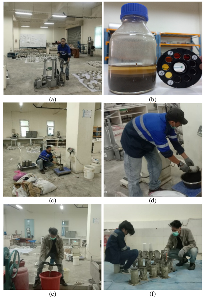
Fig. 1. (a) Sand aggregate screening process, (b) checking the sand aggregate content using a color disc tool, (c) weighing sand aggregate using a funnel, (d) weighing crumb rubber aggregate for mortar specimen mix, (e) mixing normal mortar and crumb rubber mortar variations, (f) mortar mold preparation process on a cylinder.
