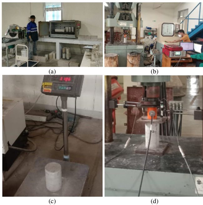
Fig. 3. (a) The process of heating the cylinder in an oven at a temperature of 150 °C, (b) preparation of tool settings and cylinder testing using UTM and LVDT tools, (c) the process of weighing cylindrical samples before the testing process using a weighing tool, (d) compressive strength testing process using UTM and LVDT.
