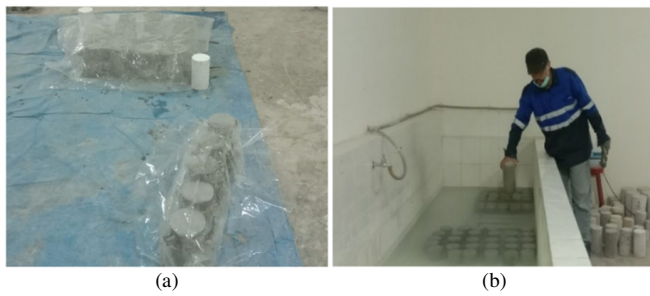
Fig. 2. (a) Mortar specimen treatment with a cylinder using plastic on the first day in a water bath, (b) on the second day, the mortar specimens were removed from the cylinder for curing in a water soaking bath.
