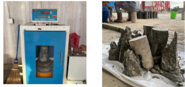
Fig. 3. Compressive strength testing.
