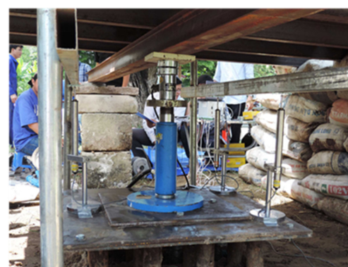
Fig. 3. Setup of the measuring apparatus on the test pile group to record the loads, movements, and deformation of each instrumented pile.
