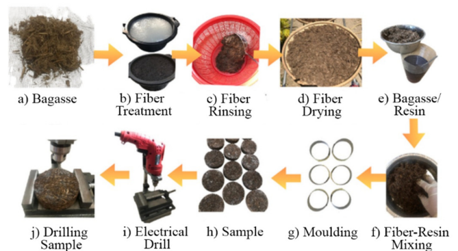
Fig. 2. Bagasse composite and sample preparation.
