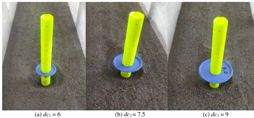
Fig. 13. The scour hole formed by different collar external diameters at 45 min.
