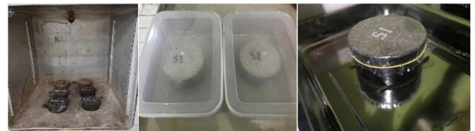
Fig. 2. Sorptivity Setup: oven-drying; sealed conditioning; and sealing of all faces except the exposed face (shallow water contact).
