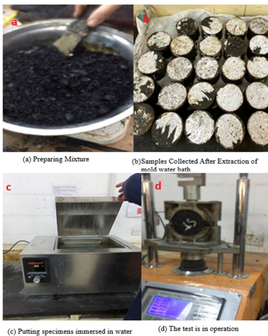
Fig. 3. Testing of Marshall specimens.
