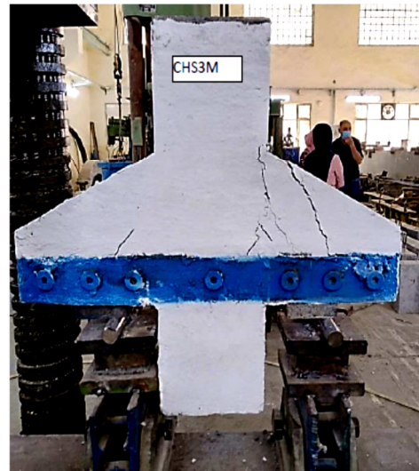
Fig. 4. Corbel patterns of cracks after testing.
