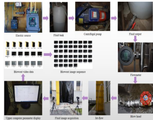
Fig 6. Flow of video acquisition of simulated blowout fluid
