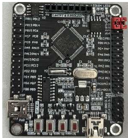
Fig 3. STM32 minimum system
