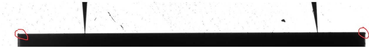
Fig 13. Contact illustration between the blade and tungsten steel needle
