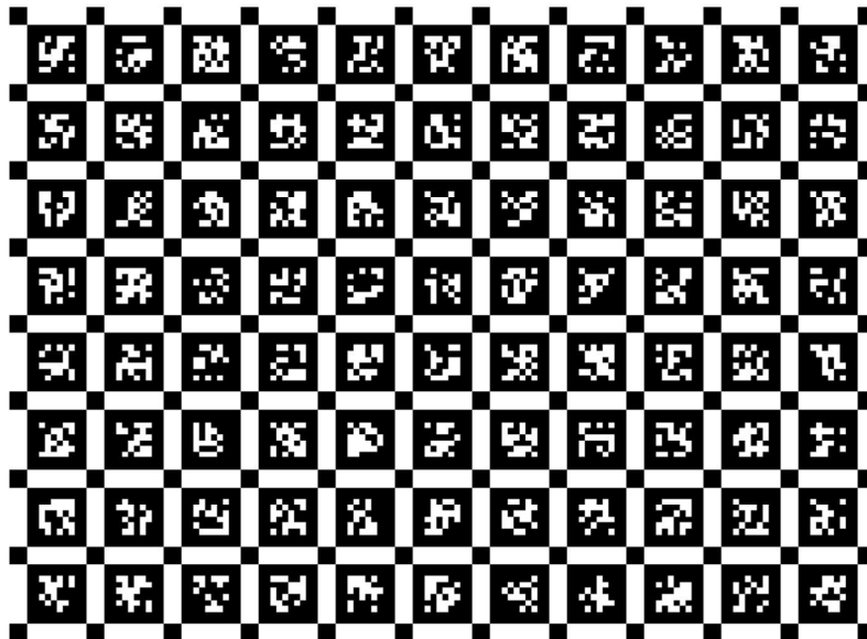
www.calib.io | 8x11 | Tag Size: 12 mm | Tag Spacing: 3.6 mm | Dictionary: t36h11.
