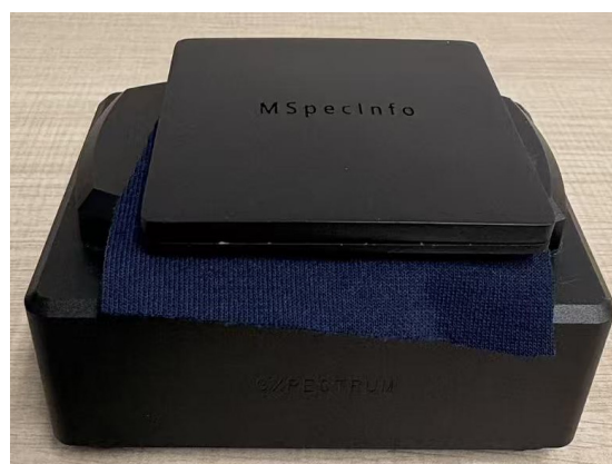
Fig 2. Near infrared spectroscopy data acquisition device
