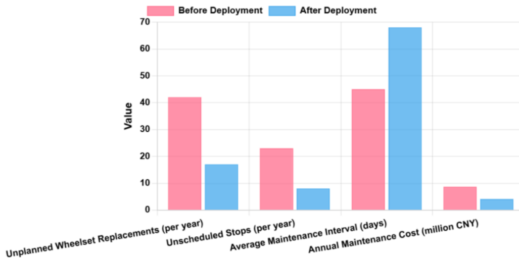
Figure 7. Comparison of wheelset maintenance data before and after deployment of the multimodal fusion system
