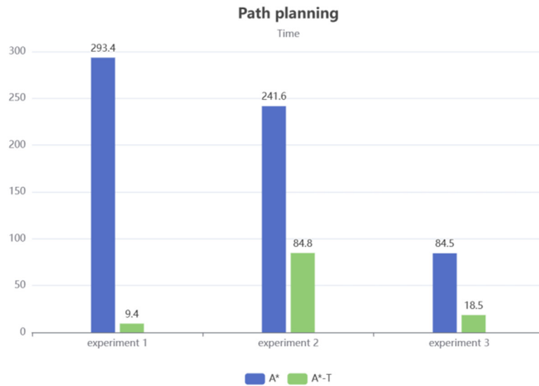
Figure 3. Bar Chart of Path Planning Experimental Results for A* Algorithm and A*-T Algorithm
