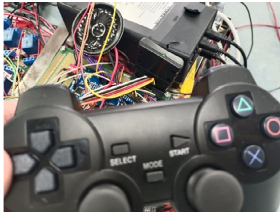
Fig 5. Remote Control Handset for Remote Operation
