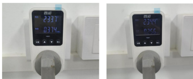
(a) Hot air 30°C energy consumption (b) infrared hot air 35°C energy consumption
