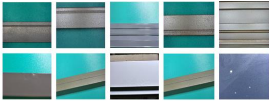
Figure 6. Pictures of aluminum defect categories
