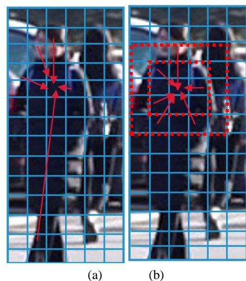
Figure 1. The sight of CNN and transformer. (a) CNN aggregates relational features from pixels locally and focus on small regions. (b) Transformer explore long-range dependencies, thereby calculating attention mechanisms globally.
