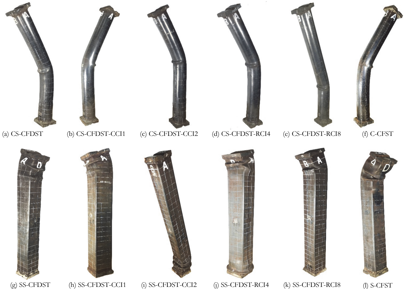
Figure 7: Failure modes of composite columns.
