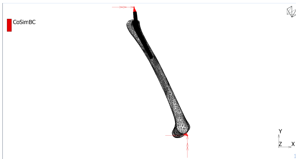
Figure 4: Boundary conditions for the FEM model.
