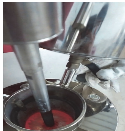
Figure 8: Stirring of Molten Metal.
