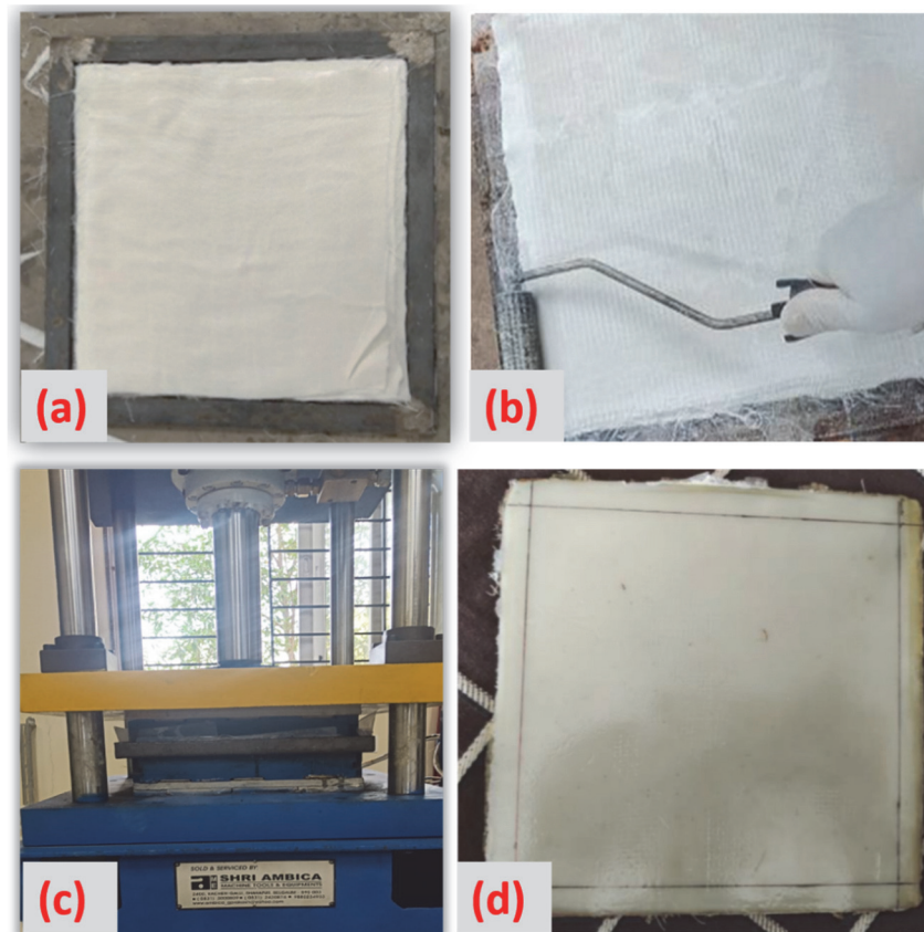
Figure 3: (a) Steel mold with bamboo fiber (b) Wetting of fibers (c) Compression molding (d) Composite plate.
