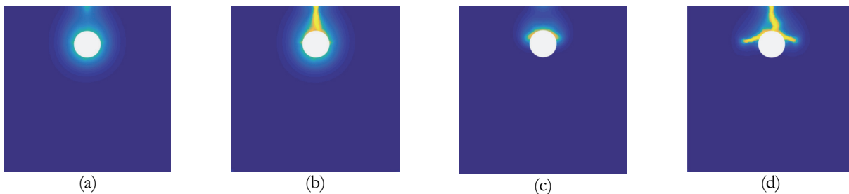
Figure 4: Crack development on the 1-D20 cross-section and c=15\text{mm} : (a) crack nucleation and (b) complete crack development due to the uniform corrosion; (c) crack nucleation and (d) complete crack development due to the non-uniform corrosion.
