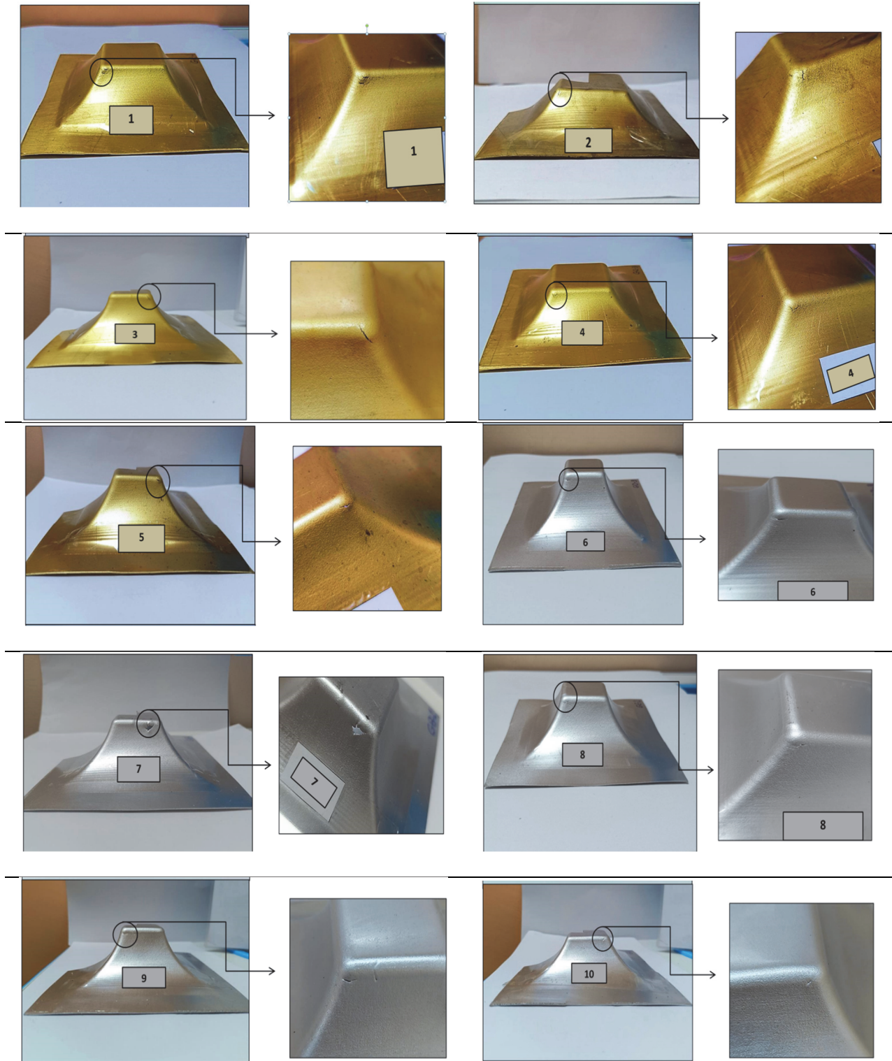
Figure 3: The resulting experimental specimens from the single point incremental forming process with their fracture zones.
