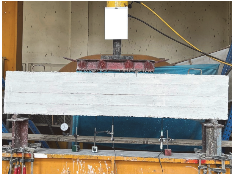
Figure 3: Four points loading that transfer from load cell to beams.
