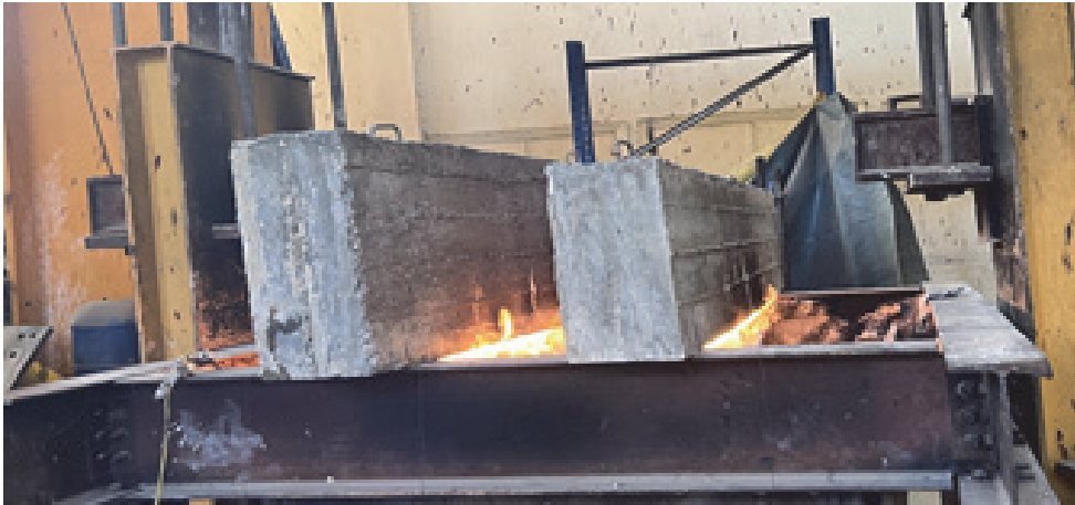
Figure 5: Specimens during the fire.
