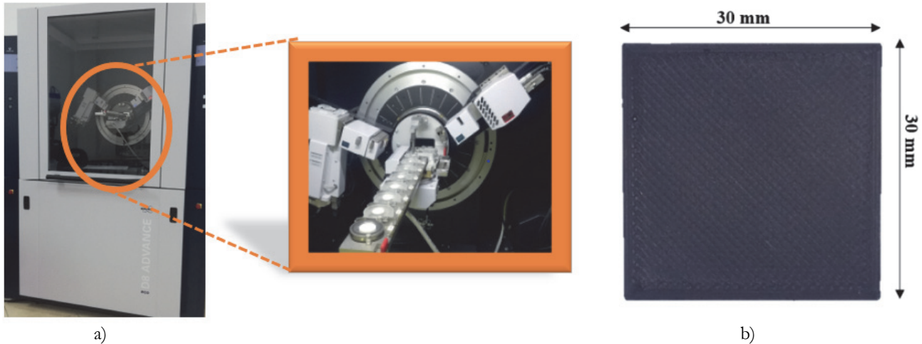
Figure 1: a) BRUKER-AXS D8 diffractometer, b) Sample of PLA-CB printed in square form for X-ray testing.
