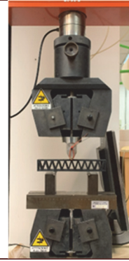
Figure 5: Sketch and picture of experimental setups: (a) tension test on DB samples; (b) tension test on beam samples (c) three-point bending test on beam samples.
