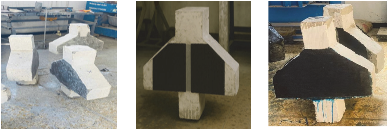
Figure 3: Mechanical grinding and installing of CFRP sheets.
