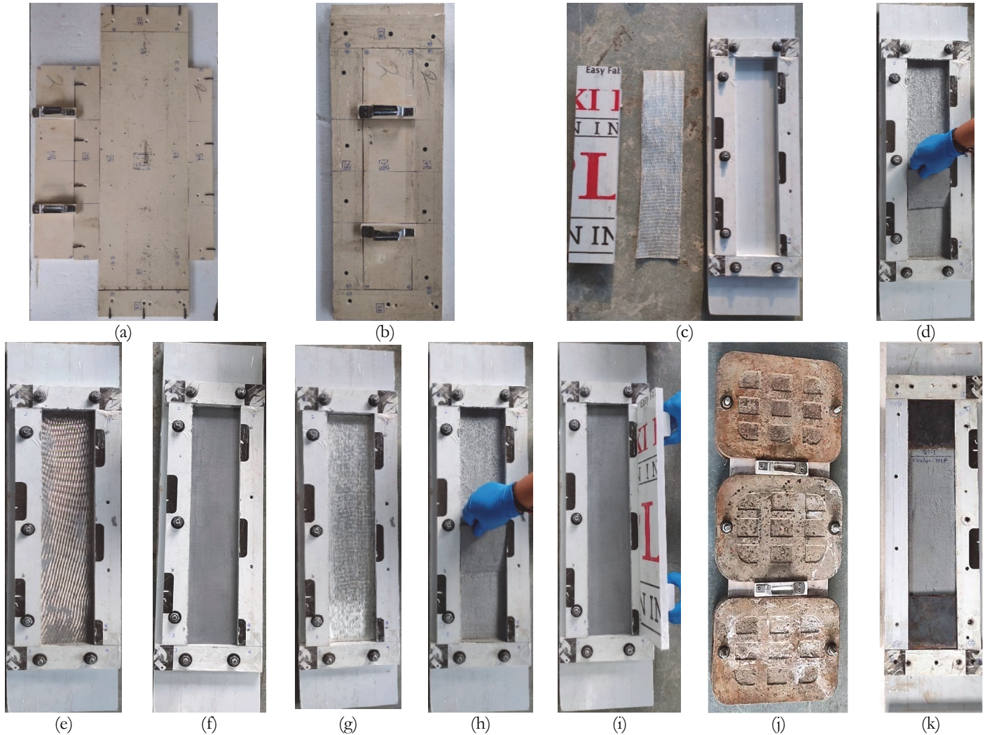
Figure 4: Illustrative photographs of step-wise procedure for development of hybrid GFRP-SSWM wrap.
